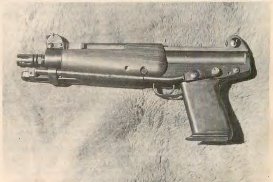
ABOVE: First prototype of Johansson's PC-80 in .221 Fireball caliber, left-hand view, with stock extended and 16-inch barrel installed. RIGHT: PC-80 with stock folded forward in stowage position. Note location of sling swivels. LOWER RIGHT: Short-barreled version of PC-80 with stock folded. There was no selector switch on prototype sent to author.
